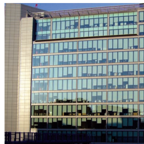
When solar shading is not designed as part of the architecture it is almost inevitable that the occupants will take matters into their own hands, often spoiling the architectural concept.
