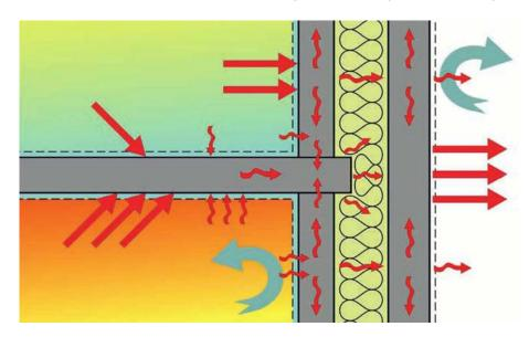
The traditional U-value calculation models a simple, linear flow of energy from the internal air to the external air by conduction alone (accounting for the resistance of a stagnant air boundary layer). In fact, to represent the true picture, we ought to account for absorption and emission of energy by radiation, differential conduction into the internal face at high and low levels due to stratification, and for three dimensional flows within the construction
