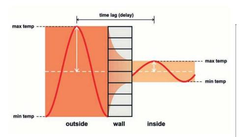
Diurnal variations in external temperature are attenuated by building envelopes to the extent that they contain thermal mass to partially absorb the energy flow. This results in a dynamic insulation property known as decrement
