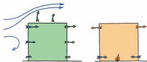
Natural air movement in buildings will be driven either by wind pressures (left) or stack pressure generated by a heat source raising the internal temperature (right). The wind and stack effect will act in opposition in parts of the building and reinforce flows in others. In low-rise buildings, wind pressure will tend to dominate, but in high-rise buildings the stack pressures can exceed the wind pressure.
