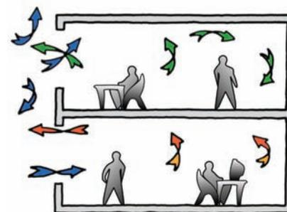
Single-sided ventilation can be effective in shallow-plan spaces with opening windows. The air movement is driven either by turbulence of the wind at the face building (above top) or by internal heat gains driving stratification and displacement ventilation (above bottom).
