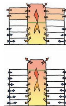
In atrium buildings, ventilated by stack effect, it is important to consider the position of the neutral plane (green). Above the neutral plane air will flow outwards from the stack and if this is allowed to happen at occupied floors, they will overheat (top). Changing the atrium geometry and the balance of high- and low-level openings moves the neutral plane above the occupied levels (bottom).
